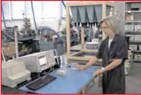
Final test with network analyzer
